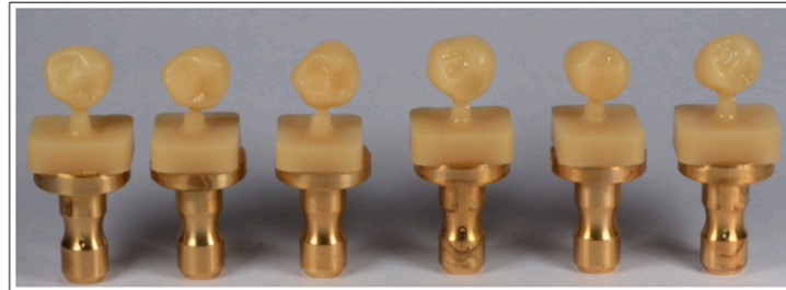
Figure 5. Ceramic crowns after milling.
