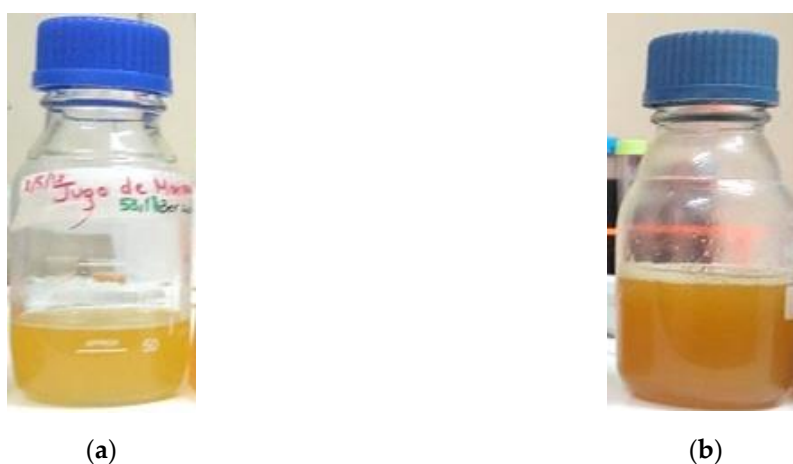
Figure 3. Samples of apple juice: (a) fresh juice; (b) cryoconcentrated sample (3rd cycle).
