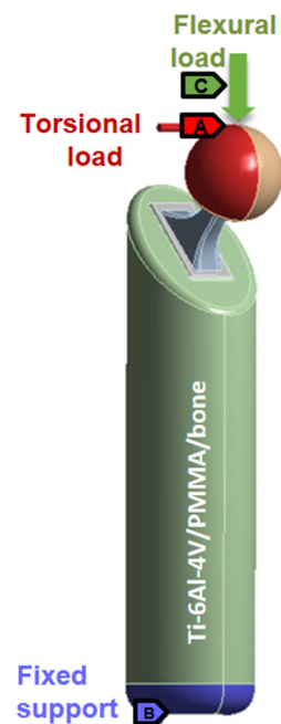
Figure 4. Load distribution for structural analysis.
